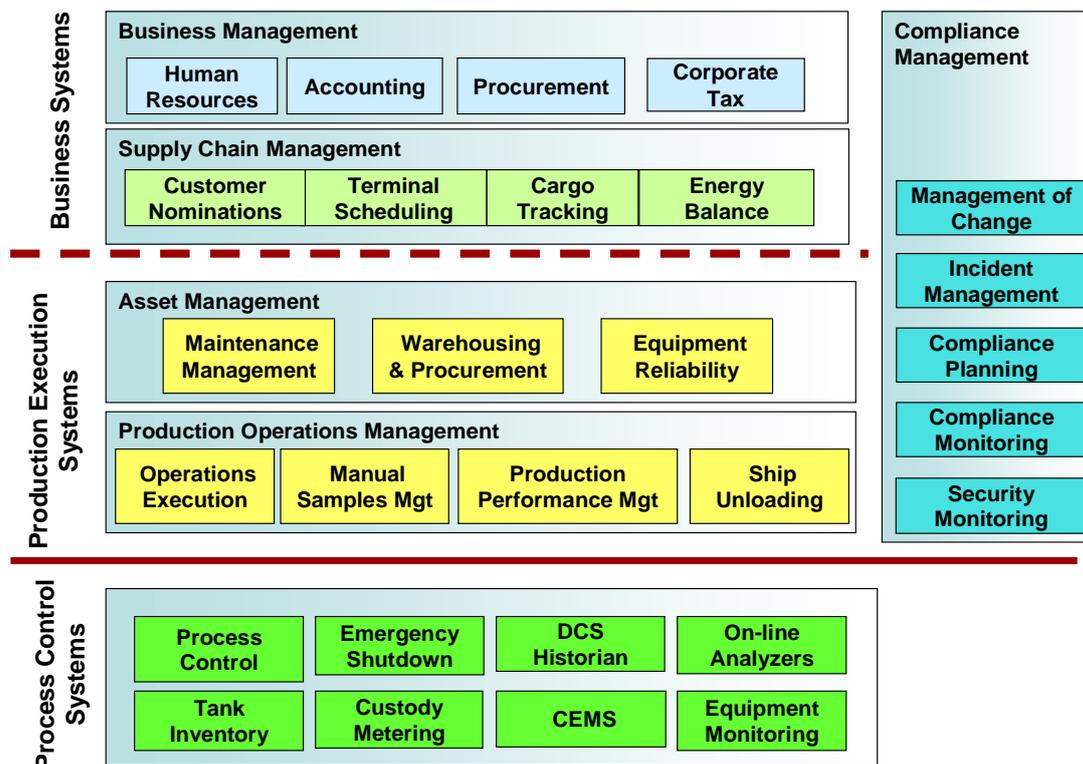
**Figure 4. Typical Terminal Functional Architecture (PCS and TIMS)**
